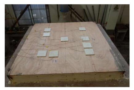
Photo No. 10 **Unexposed Surface after Fire Endurance Test (30 minutes)**
