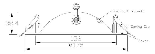
Dimension Drawing of Model FR-LED-6-S15W-5CCT-FG-\*\*
