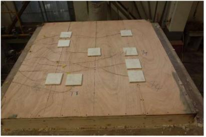
Photo No. 9 **Completed Assembly - Unexposed Surface before Fire Endurance Test**
