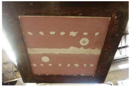
Photo No. 8 Completed Assembly - Exposed Surface before Fire Endurance Test
